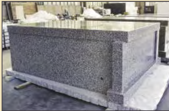
16. Two vents are included on each side of the mausoleum.
